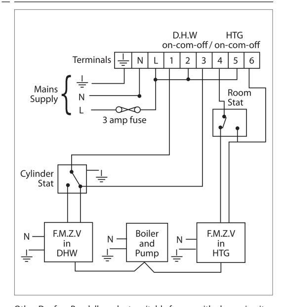
Other Danfoss Randall products suitable for use with above circuit:-AT cylinder thermostat; RMT room thermostat.
