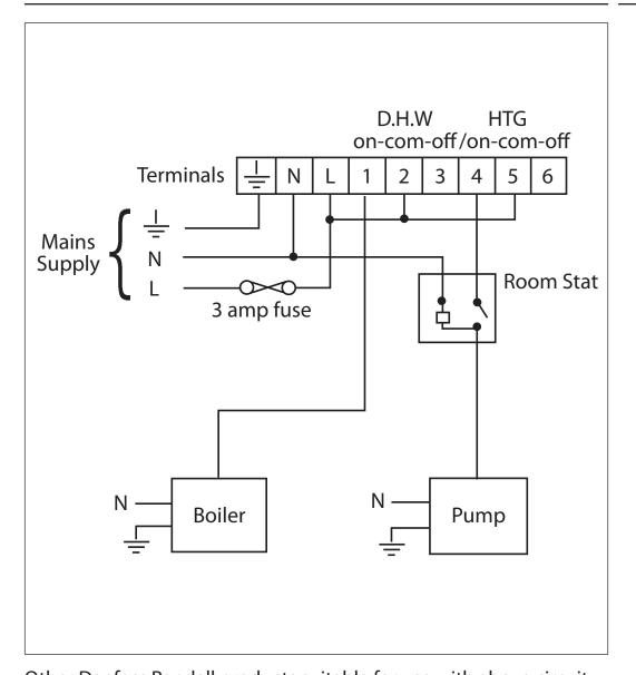
Other Danfoss Randall products suitable for use with above circuit:-RMT room thermostat.
