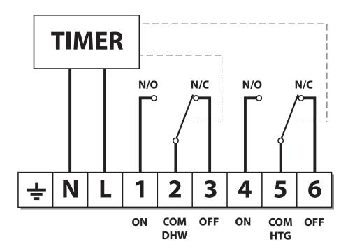
**NOTE**: For mains voltage applications links must be fitted between terminals L, 2 and 5.
